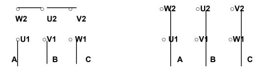
If the motor's junction board has 3 terminals (or 3 direct leads), marked with U, V, and W, only press A-U, B-V, and C-W.
